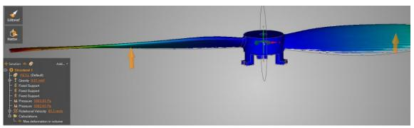
Fig. 6. Deformation of the propeller blade
