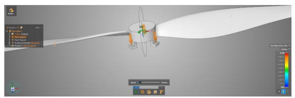
Fig. 5. Boundary conditions of propeller legs
