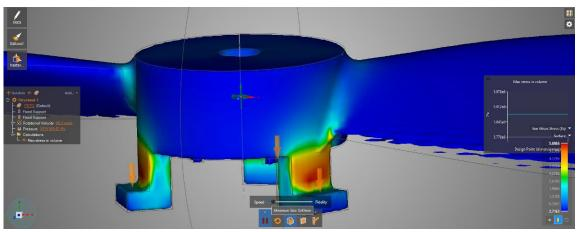
Fig. 9. Maximum stress in propeller legs for PETG
