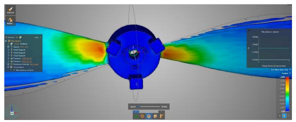
Fig. 8. Maximum stress in propeller blades for PETG
