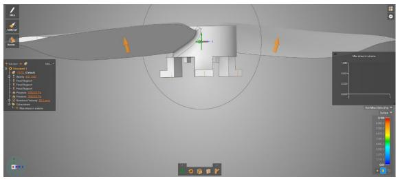
Fig. 4. Forces applied on blades of the propeller
